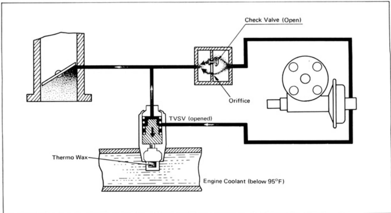
Fig. 5-2 Spark Delay System Operation (Coolant Temperature Below 95°F)
