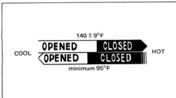
Fig. 5-5 TVSV Operation Temperature Range
