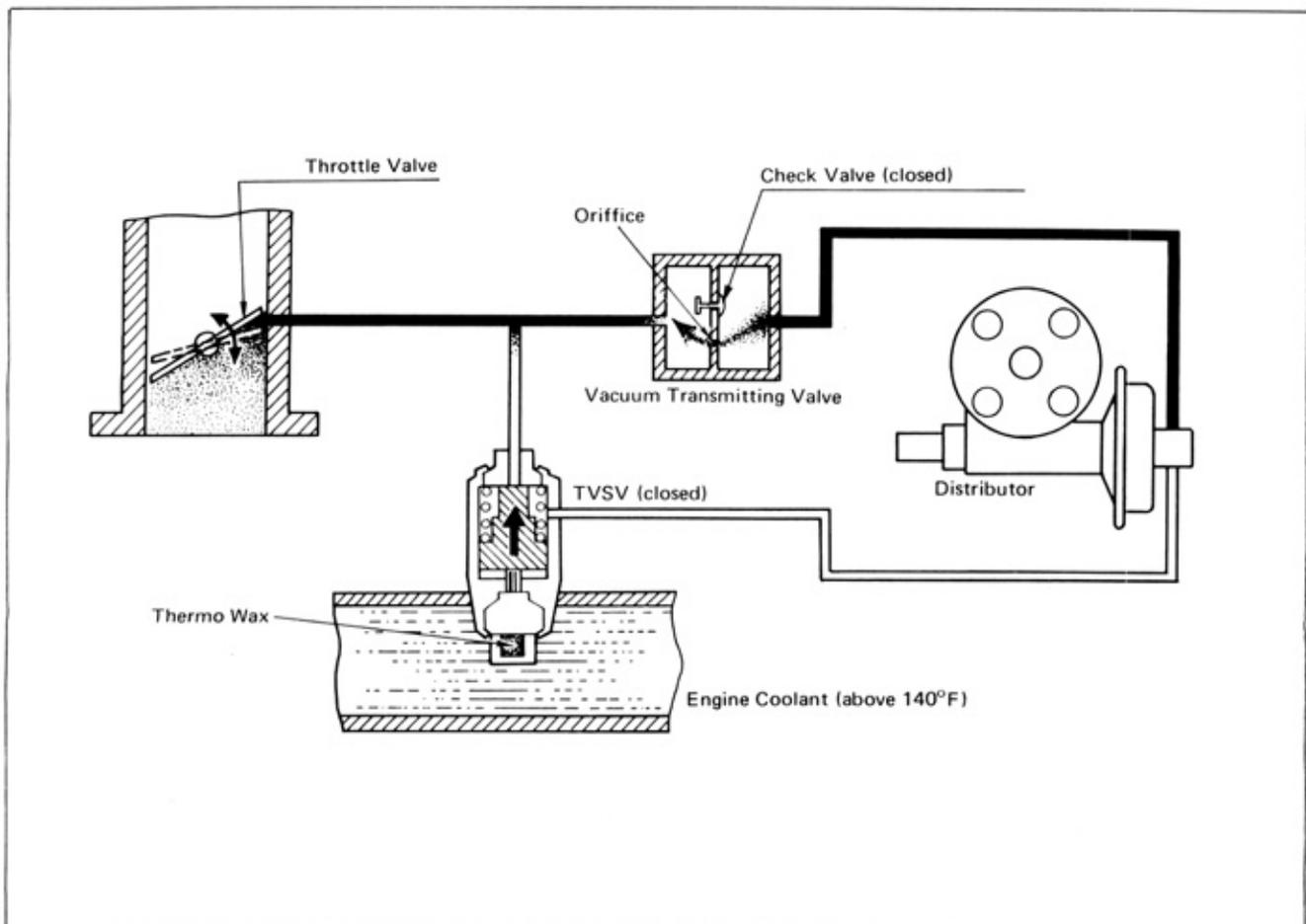
Fig. 5-1 Spark Delay System Operation (Coolant Temperature Above 140°F)
