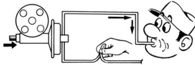
Fig. 5-7 Distributor Inspection
