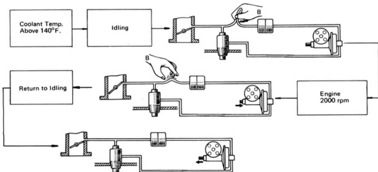
Fig. 5-9 Vacuum Transmitting Valve Inspection
