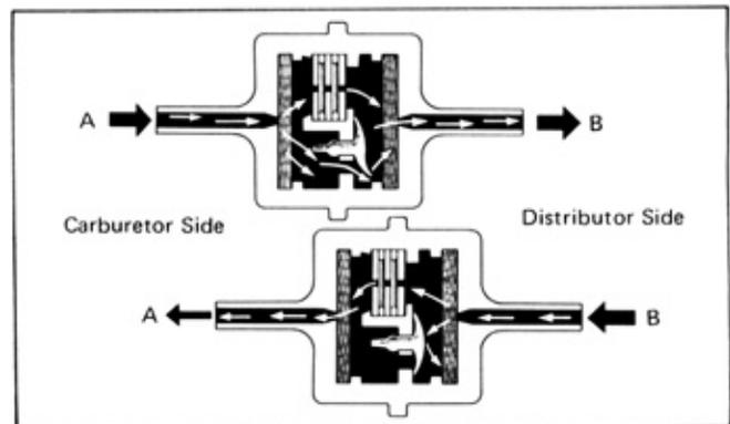
Fig. 5-3 Vacuum Transmitting Valve
